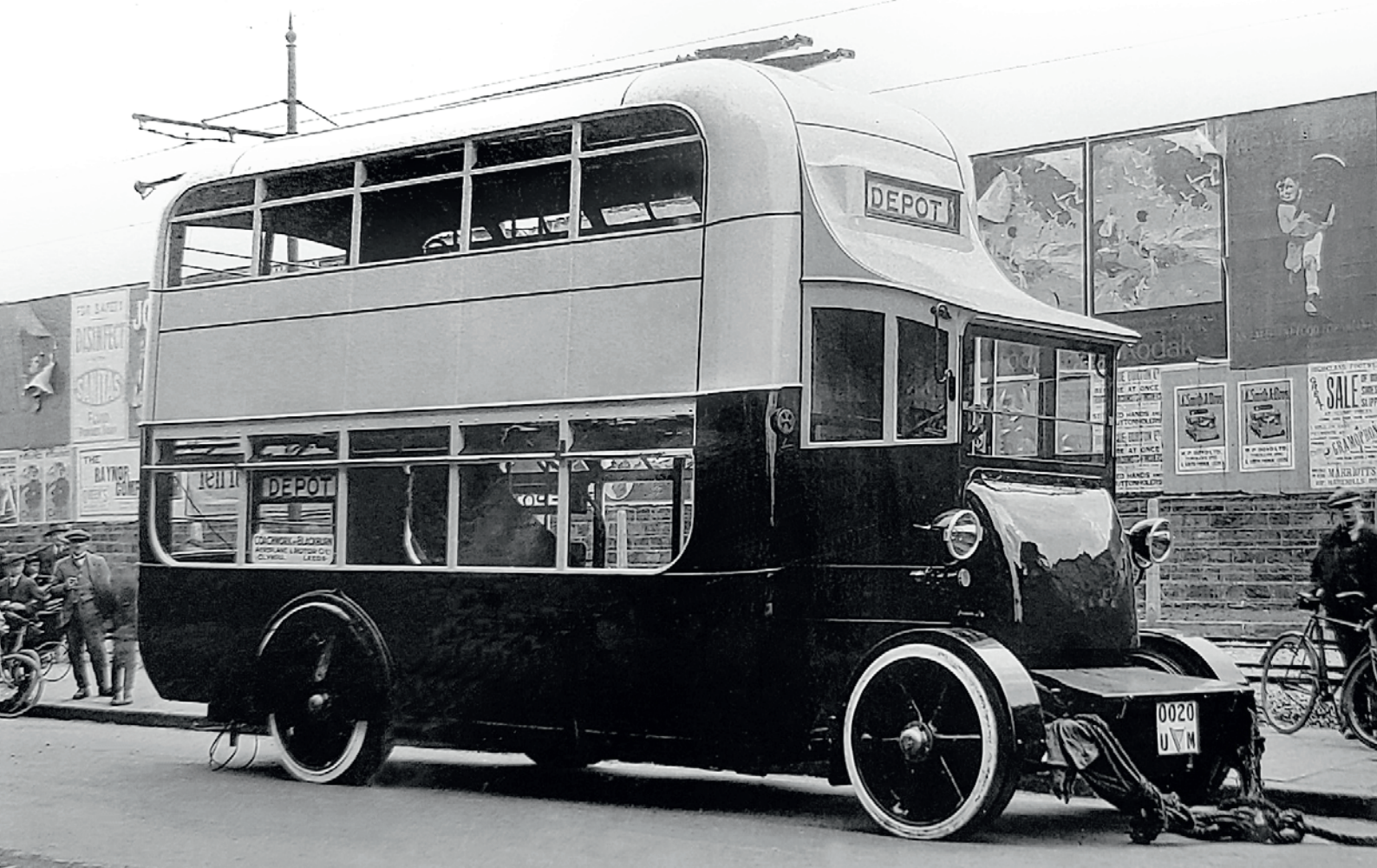
Before embarking on its tour of the country, the Trackless Cars low-height (13 feet 10 inches) demonstrator was tested on the Leeds system on 17 June 1922 and this photograph is one of a number taken on that occasion. Before it was acquired by Leeds Corporation in December 1923 an upper deck windscreen replaced the destination indicator.
