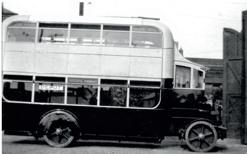
The Trackless Cars demonstrator parked at Coventry's Priestley's Bridge tram depot looking a little less pristine than it did in Leeds before its journey around the country. Note the position of the bamboo retrieving stick on hooks attached to the window pillars. Travel Lens Photographic
